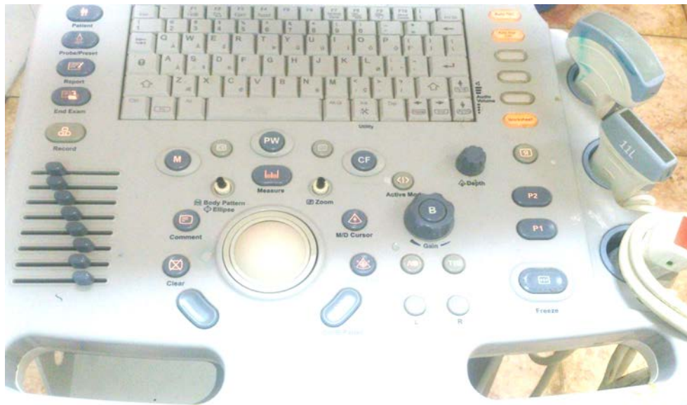
Fig. (17):- General Electric (GE) ultrasound portable device control pannel
